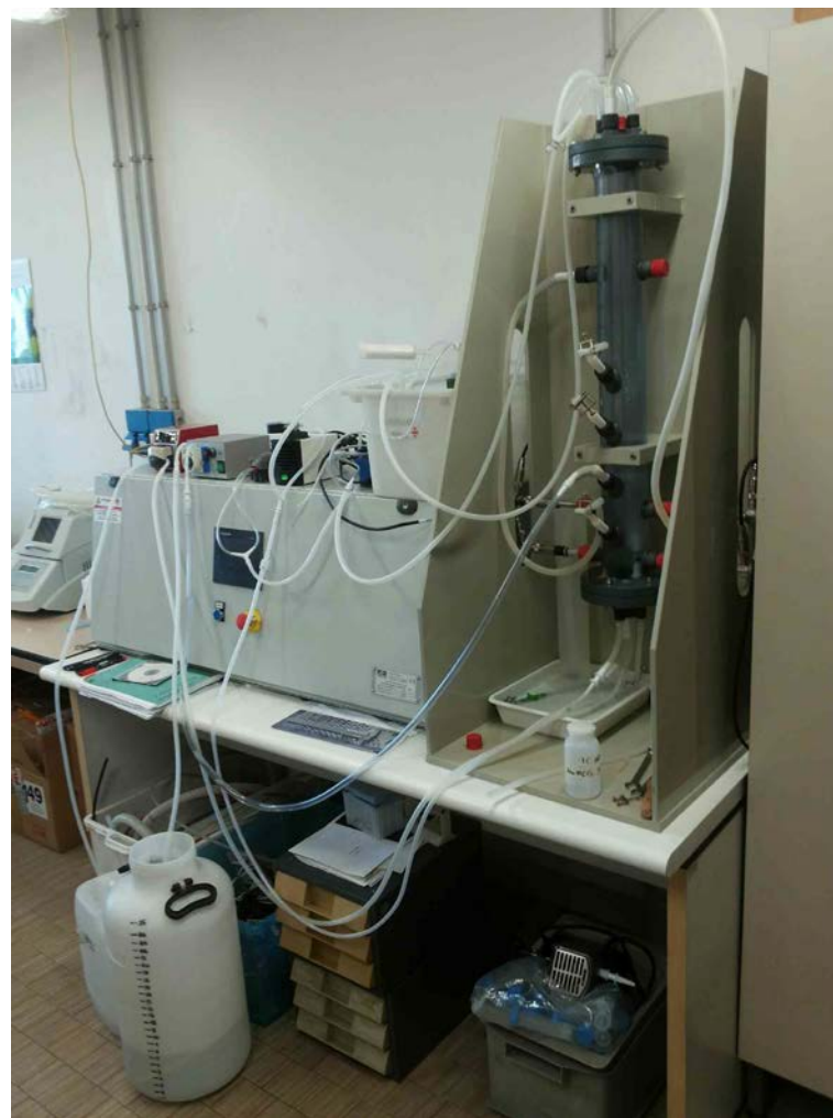
Impianto SBR (Sequencing Batch Reactor) STRUMENTATO
